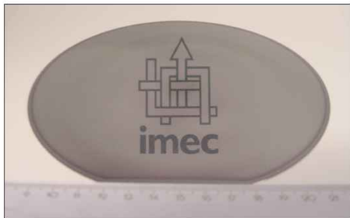
Figure 1: A 150mm GaN HEMT on a silicon wafer.
