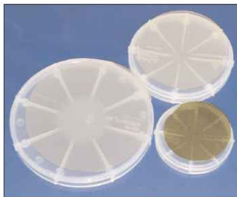
2", 3", and 4" AlN-on-SiC wafers. Thick AlN layers are deposited on electrically conducting SiC by HVPE.
